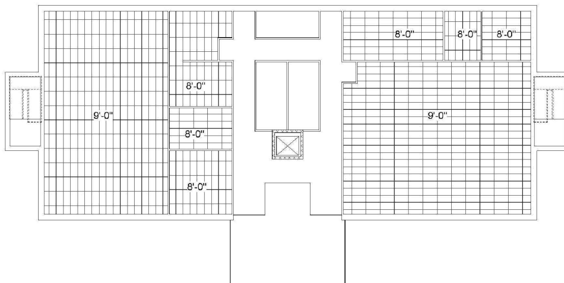
FIGURE 7-2.5 Level 1: Ceiling Grids
