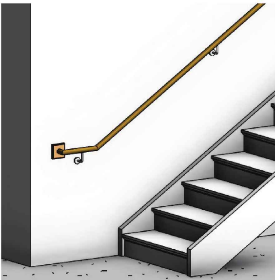
FIGURE 5-4.32 Handrail only with supports at 6'-0" O.C. max.
