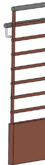
FIGURE 5-4.12 Railing with stringer
