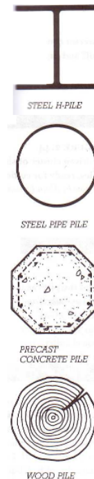
FIGURE 2.42 Cross sections of types of piles. Precast concrete piles may be square or round instead of the octagonal cross section shown, and may be hollow in the larger sizes.
